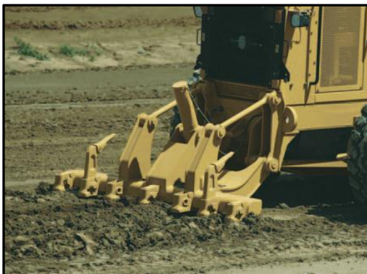
Figure 22. Grader ripping compacted soil.
