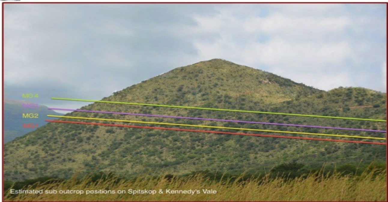
Figure 2: View of Spitskop and Kennedy's Vale in an easterly direction, MG1, MG2, MG3 and MG4 Package are indicating sub-outcrop position as well as dip direction.
