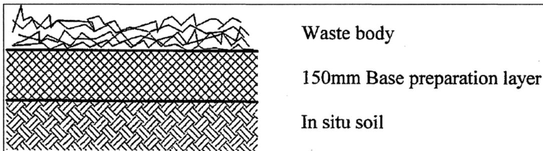
**Figure 11.** Class D Landfill Engineering Design.
