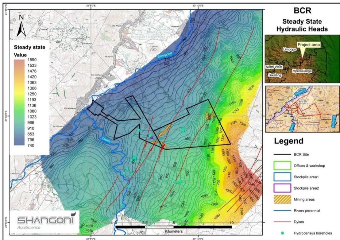
**Figure 7.** Steady state hydraulic heads, hydrocensus boreholes and direction of groundwater flow depicted by arrows (Delta-H, 2016).
