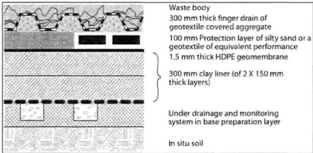
**Figure 10.** Class C Landfill Engineering Design.
