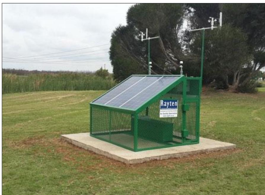
**FIGURE 6-2: EXAMPLE OF PM10/PM2.5 MONITORING STATION SUITABLE FOR REMOTE LOCATIONS.**
