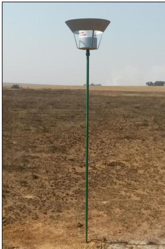
**FIGURE 6-1: EXAMPLE OF A SINGLE DUST FALLOUT BUCKET UNIT WITH A WINDSHIELD.**
